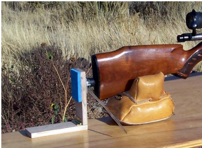
Rifle set up for making recoil measurements. ( LoadForce-250 module not shown for clarity.)
