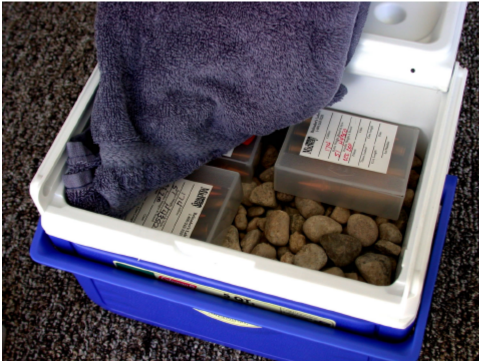
Test cartridges packed for the test. A few pounds of river rock in the bottom of the cooler regulated the temperature. A towel, folded on top of the ammunition boxes, provided additional insulation.
