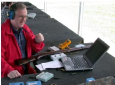
On the far left, a yellow digital thermometer used to measure barrel temperature, then the M39 rifle. The small white box between the rifle and the laptop is the Southwest Products interface. Barrel temperature is an important variable in chamber pressure, so I run most of my tests at a constant barrel temperature of 100°F. I have no idea who the fat guy is.
