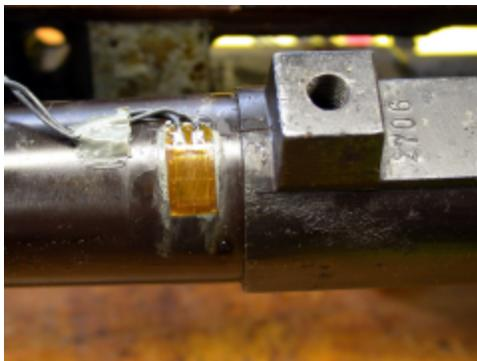
The strain gauge is glued to the barrel, at about the midpoint of the casing. The gray blob to the left is a dab of JB Weld. It prevents me from accidentally yanking the wires off the strain gauge.
